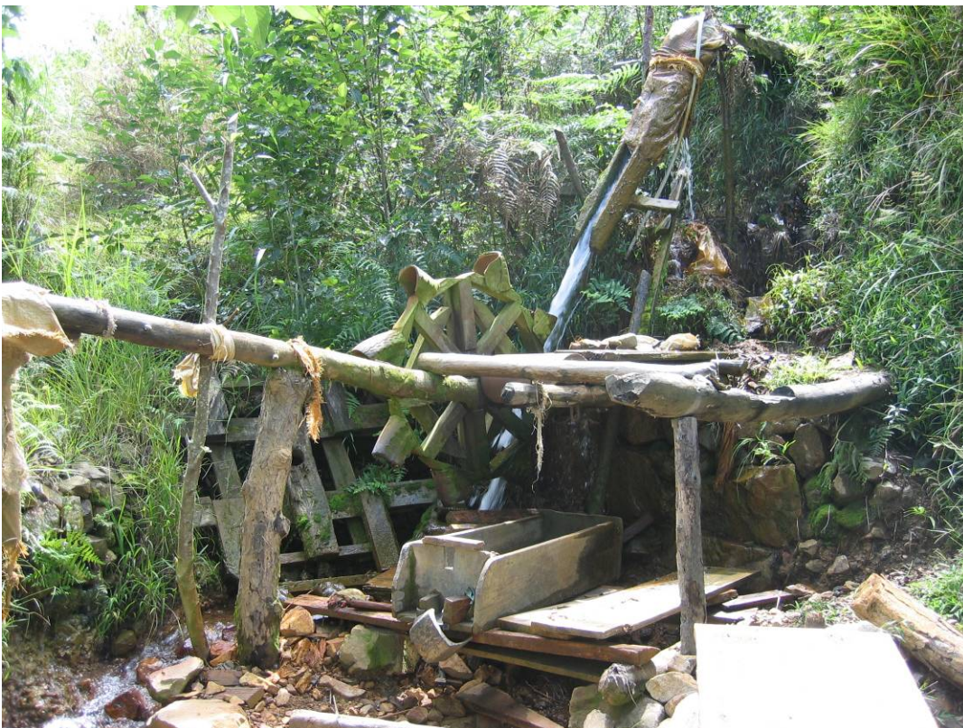
A water powered ball mill and sluice box used by artisan miners to the west of Hermans Find
